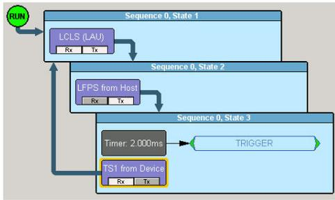
LeCroy's USB 3.0 analyzer provides sequential state detection with independent timers in each state for identifying timing violations
