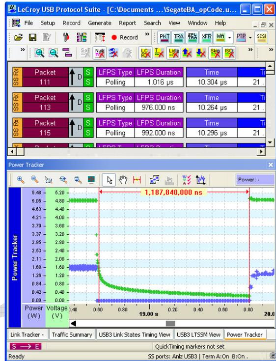
Power Tracker™ monitors  $v_{BUS}$  power draw and displays voltage graphically in a time line format
