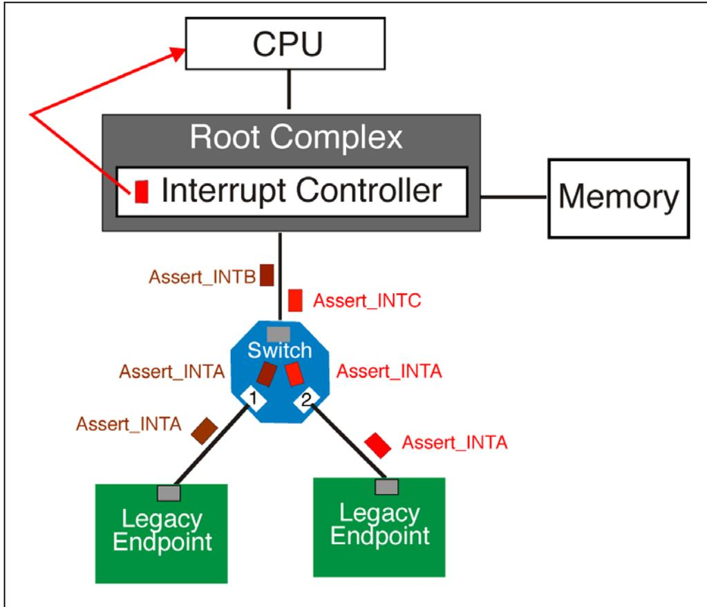
**INTx Collapsing.** In some cases two overlapping INTx messages may be mapped to the same INTx message by the virtual PCI bridge at the egress port, requiring the messages to be collapsed. Consider the following example illustrated in Figure 6 on page 23.
